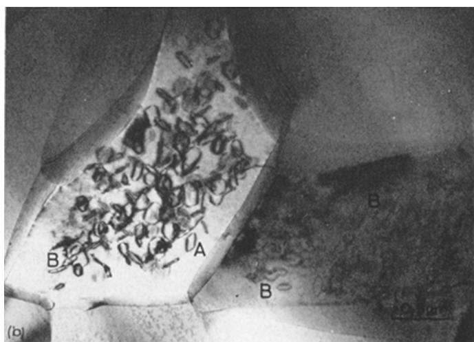
Figure 2 Defect structures in a splat-cooled Al-5.7 at. % Ag alloy. (a) A large number of black spot defects which may be either very small dislocation loops or vacancy clusters. (b) Various dislocation loops; regular hexagons, parallelograms (A) and large loops with irregular shapes (B). Loop density, 2.3 \times 10^{14} \text{ cm}^{-3} ; loop diameter (average), 1800 Å; estimated concentration of quenched-in defects, 0.7 \times 10^{-3} . (c) Tangled dislocations.
